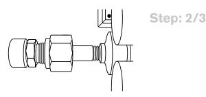
The parts MUST be tightened together prior to attachment to the paintball bottle. If the bottle adapter is connected first,  $CO_2$  gas will bleed from the bottle since the bottle does not have a shut off valve. The regulator should be in the closed position so that  $CO_2$  does not drain when the main assembly is attached to the paintball bottle.
