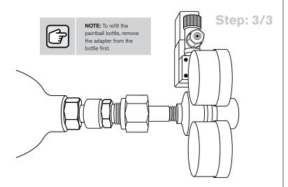
After the adapter is attached to the regulator, the main assembly can be attached to the paintball bottle.
