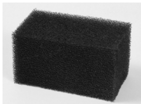
Figure 12: Mechanical filtration material
