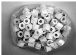
Figure 3: Biological filter material
